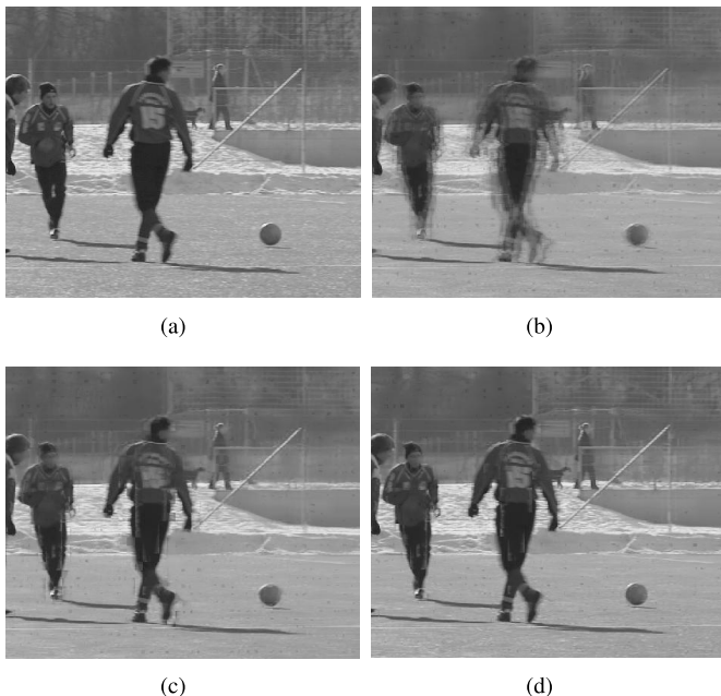
Fig. 6. Visual quality comparison for side reconstruction of Soccer 26th frame. (a) Original. (b) [12]: 2475.9 kb/s, PSPNR = 27.863 dB. (c) Proposed: 2474.2 kb/s, PSPNR = 30.172 dB, p\% = 70%. (d) Proposed: 5588.3 kb/s, PSPNR = 31.098 dB, p\% = 30%.
